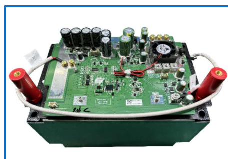
Figure 3: Naked SmartStart 100 Battery Pack and BMS Data Output
